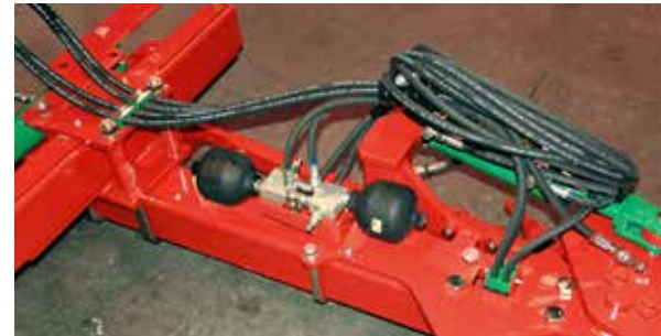
As standard, 2 accumulators are fitted to the BE plough for safe steering
