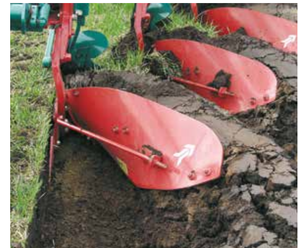
furrow profile body No. 28 working depth: 26 cm, bottom: 30 cm, width 73 cm
